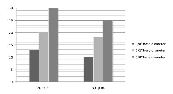
Pressure from power pack: 150 bar., Flow: 20 l.p.m., zero elevation, 2 set couplings per 10 m hose.
